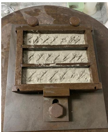
Figura 22 – Ranhuras na argamassa
